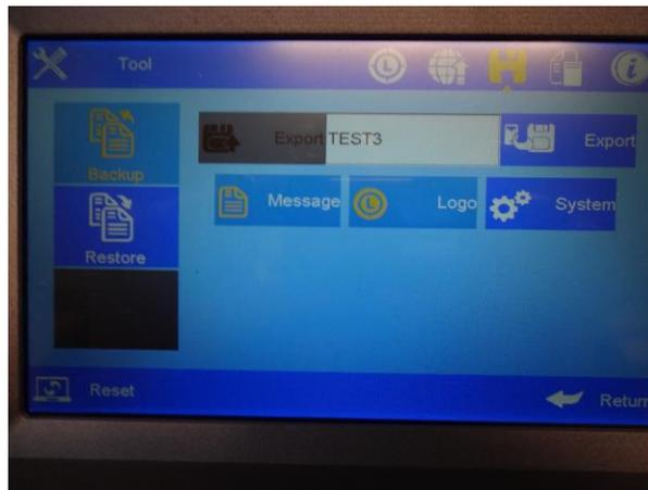
The printer will now show a progress bar and start the backup process, how long the process will take depends on the number of messages and logos that are stored on the printer. Once the backup has completed, the USB stick can be removed from the printer.
