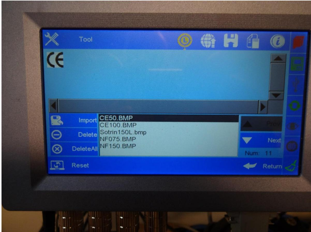
Once the USB stick has been recognised by the printer, the restore process can be started. From the **Tools/Back Up and Restore** screen, highlight **Restore** and select the desired backup folder and, ensuring no other option is selected, tap Import. A progress bar will appear and the restore process will start, once completed the printer will reboot.
