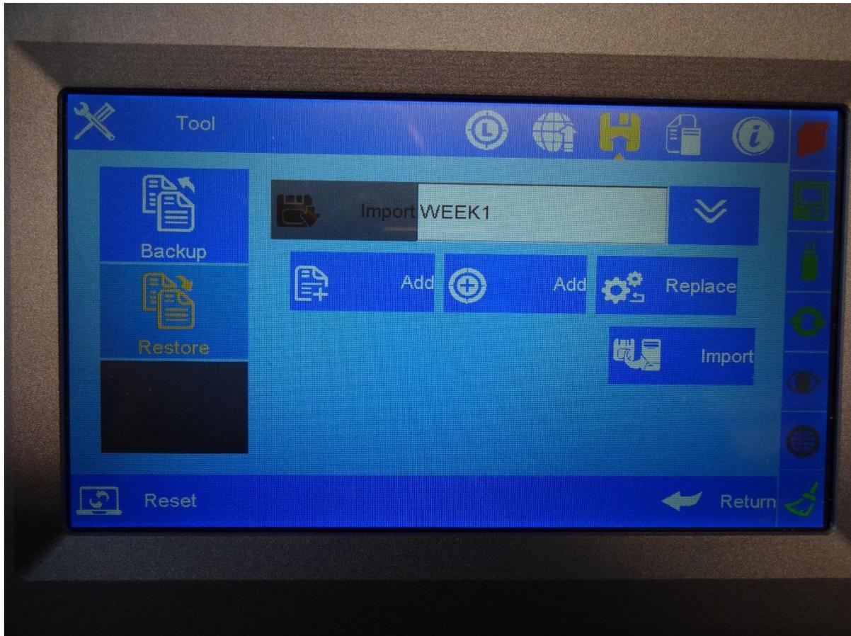
Any new messages created on the printer will need to be backed up to a new backup folder and added to the central store.
