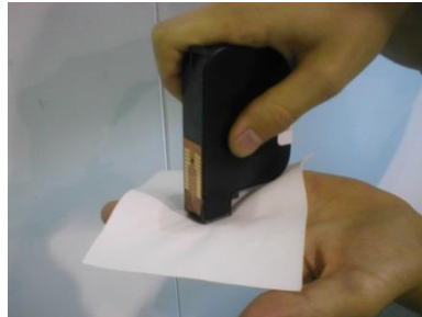
2. Put the nozzle down, and clean slowly in the direction of the nozzles.
