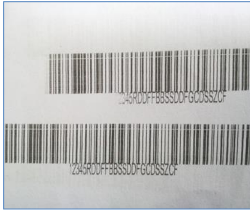
2. Missing when spray printing
